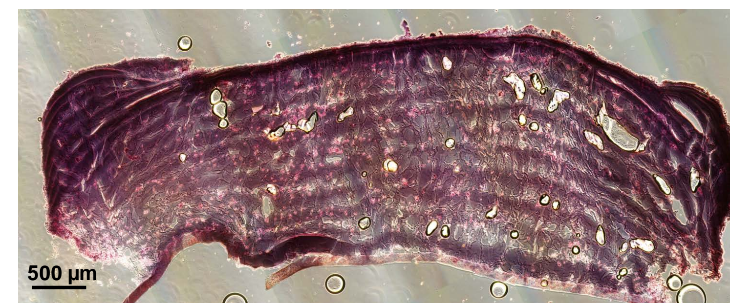
Figure 2: HE-staining of a printed skin model. A dermis equivalent containing fibroblasts was printed in a layer by layer mode. On top of the dermis a thin layer of keratinocytes was printed. The skin equivalent was cultivated for 48 hours.
